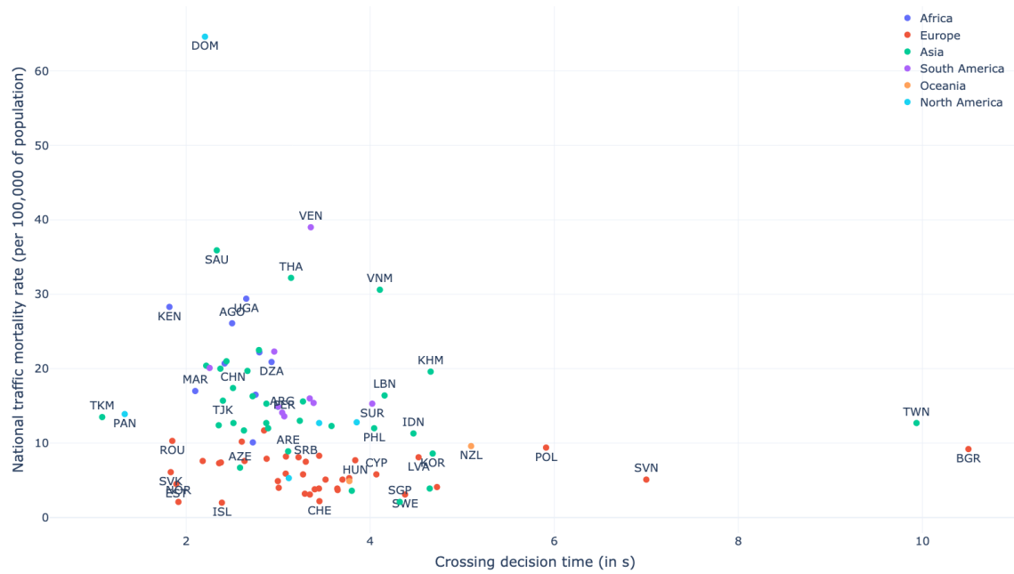
Fig. 10. Relation between traffic mortality rate and crossing decision time. Labels show the ISO-3 codes of countries.
