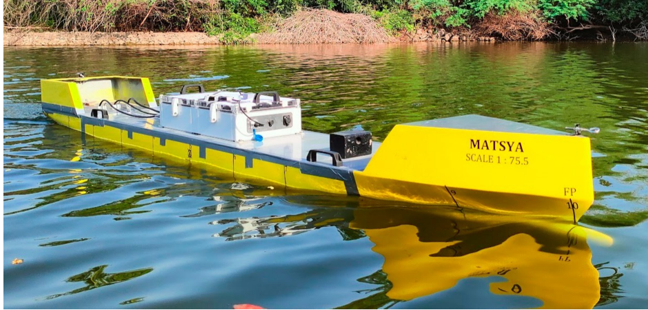
Figure 5.6: 1:75.5 scaled model of KCS
