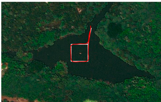
Fig. 19. Waypoints and the Trajectory: white represents the square generated by the waypoints, red represents the trajectory traversed by the vessel.
